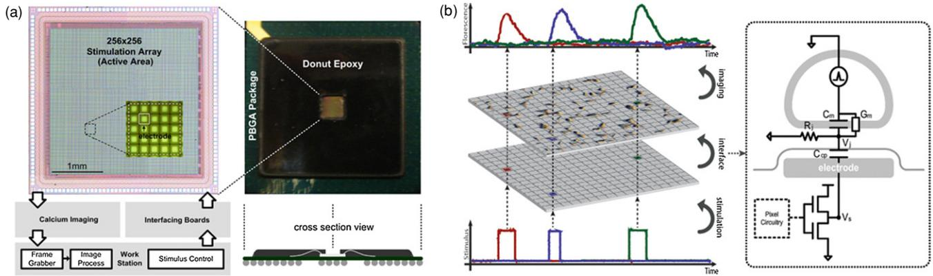
**Figure 1.** Configuration of the high-resolution MEA microsystem. (a) High-resolution stimulation microsystem platform composed of integrated CMOS MEA and optical recording microscopy. Chip package using ball grid array is shown. (b) Working principle of the microsystem. Expansion illustrates a lumped model of the neuron–capacitor–silicon interface.
