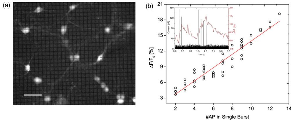
**Figure 2.** (a) Fluo-4 fluorescence of disperse culture growth on MEA surface. (b) Calibration curve correlating the number of action potential in a single burst with percent change in calcium fluorescence. The inset shows the raw trace of loose-patch electrophysiology with simultaneous recording of calcium signals. Results are taken over six cells. Scale bar equals 50  $\mu\text{m}$ .
