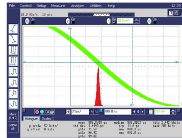
Fig. 3. Oscilloscope measurement of period jitter for clock frequency of 540 MHz. The oscilloscope measured jitter of 1.7 ps.
