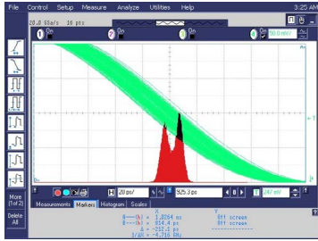
Fig. 6. Oscilloscope measurement of period jitter with jitter added by delay modulating pulse generator. f_{\text{clock}}=540 MHz.
