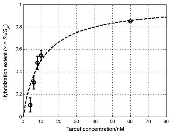
**Fig. 4.** Results of a DNA target concentration series using the active CMOS biosensor array in which the hybridization extent  $x$  is plotted as a function of the solution target concentration. The dashed line shows the Langmuir fit to this equilibrium isotherm which yields a binding constant  $K_a$  of approximately  $1 \times 10^8 \text{ M}^{-1}$ . Error bars for the four lowest target concentrations indicate the standard deviation from three separate experiments.
