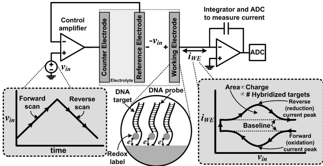
**Fig. 1.** Electrochemical quantitation of ferrocene-labeled DNA targets hybridized to probes on the surface of a working electrode using cyclic voltammetry. A potentiostat applies  $v_{in}$  to the WE interface and measures the redox current  $i_{WE}$  using an integrator and an ADC. The shape of  $i_{WE}$  as a function of  $v_{in}$  is characteristic of the response from an electroactive surface species.
