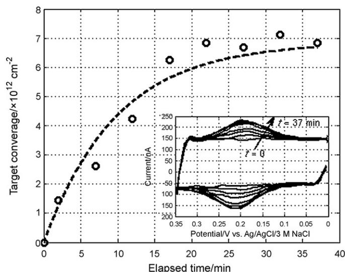
**Fig. 5.** Real-time sensing of DNA probe-target hybridization at one  $100 \mu\text{m}$  WE in which a CV scan is run every 5 min. The measured data is fit to a first-order rate equation (dashed line) following Langmuir kinetics. Inset shows the results from each CV scan over time.
