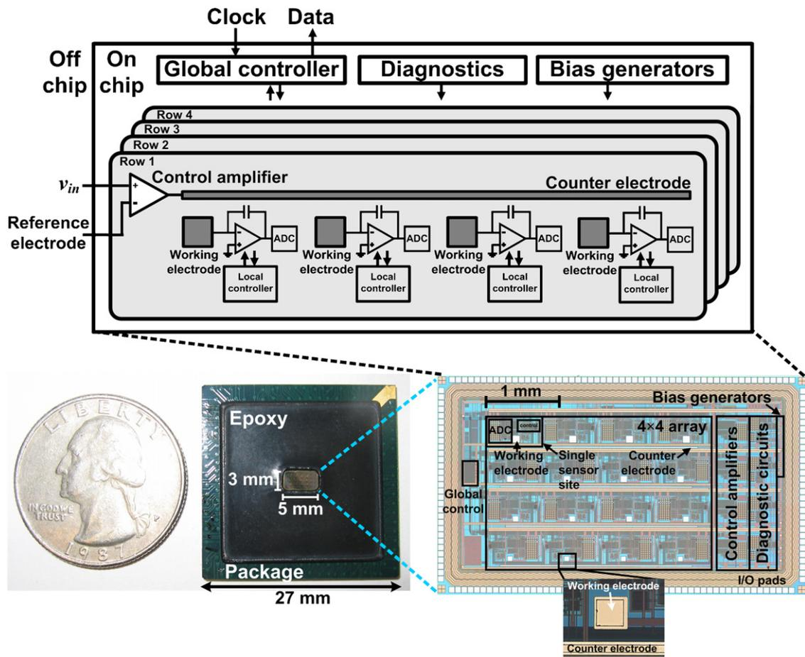
**Fig. 2.** The active biosensor array for DNA detection has been designed using a  $0.25\ \mu\text{m}$  CMOS technology, measures  $5\ \text{mm} \times 3\ \text{mm}$ , and contains potentiostat electronics with sixteen sensing sites, each having an integrated ADC to measure currents produced by electrochemical reactions occurring at the on-chip WEs. The overall system architecture, chip surface with a magnified view of a WE and CE after Ti–Au deposition, and chip packaging are shown.
